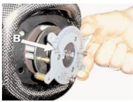
2) Remove the lampholder assembly (B).
